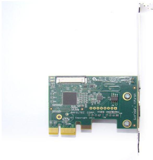
Figure 3: x1 PCI Express Host board (bottom view)
